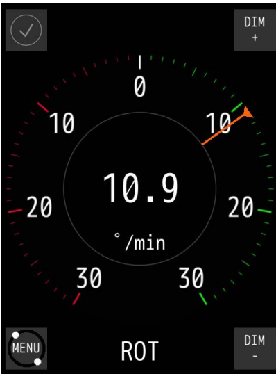
Figure 15: Main Screen AlphaTurn
